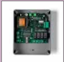
RR.4WBV RR.4WBV24 433,92Mhz 4-channels receiver rolling code. It is programmable through digital display. 230 Vac power supply mod. RR.4WBV and 24 Vac/dc mod.RR.4WBV24. Advantage system compatible. It works also by battery, 12Vdc with self-rechargeable circuit. Max. 4 relays output up to 5A
