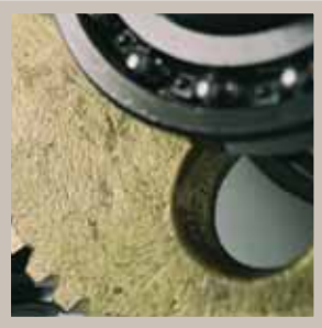
Reduction unit made of bronze gear
