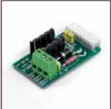
DA.RB Battery charger card for DA.S04
