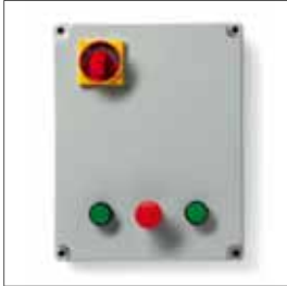
START/THINK control units with open, close, stop buttons with self-hold and three-pole door-blocking switch incorporated in the control panel. Resistant box for use in industrial environments, degree of protection IP 55. Technical features on page 159
