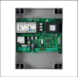
Control panel suitable for one 230Vac single phase operator up to 1500W or 400Vac 3-phases operator up to 2.200W. Built-in display for programming the functions. It is prepared with a plug-in connection for radio receiver Technical features on page 158
